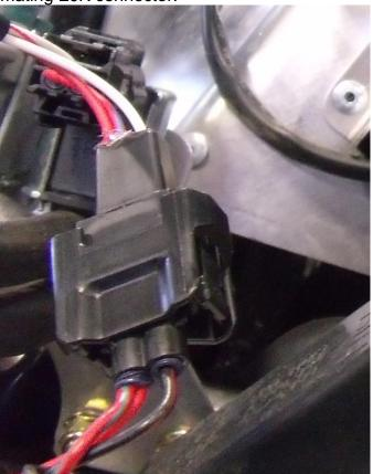
14. The EJK harness will have 2 pins without a connector on them. One will have a Red wire and the other will have a White with a Red Stripe. These will plug into the stock solenoid connector from step 10.
