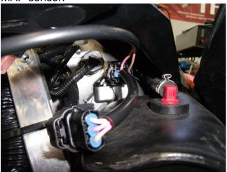
8. Locate the Waste gate control Solenoid.
