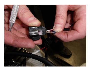
11. Once pins are removed located the black connector on the harness that has no wires inserted.
