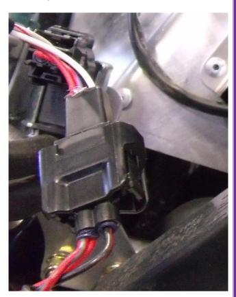
Once pins are inserted push blue pin lock into connector.
