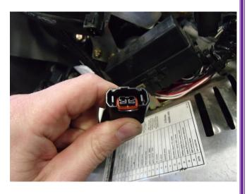
12. The above connector will plug back into the EJK mating connector. The Pins that were remove from the stock solenoid connector need to be inserted into this connector.
