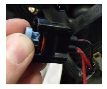
13. Plug the assembled connector into the mating EJK connector.
