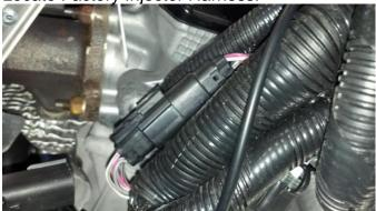
5. Plug matching EJK Harness into Factory injector Harness.
