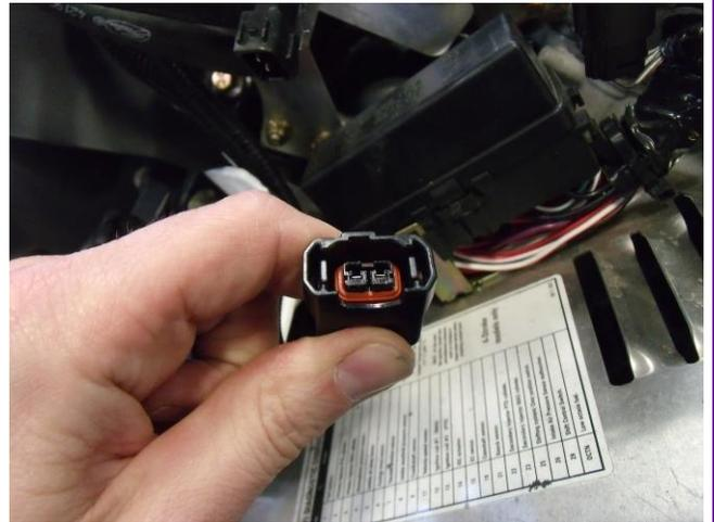
12. The above connector will plug back into the EJK mating connector. The Pins that were remove from the stock solenoid connector need to be inserted into this connector.
