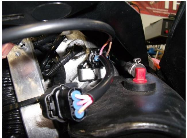
8. Locate the Waste gate control Solenoid.
