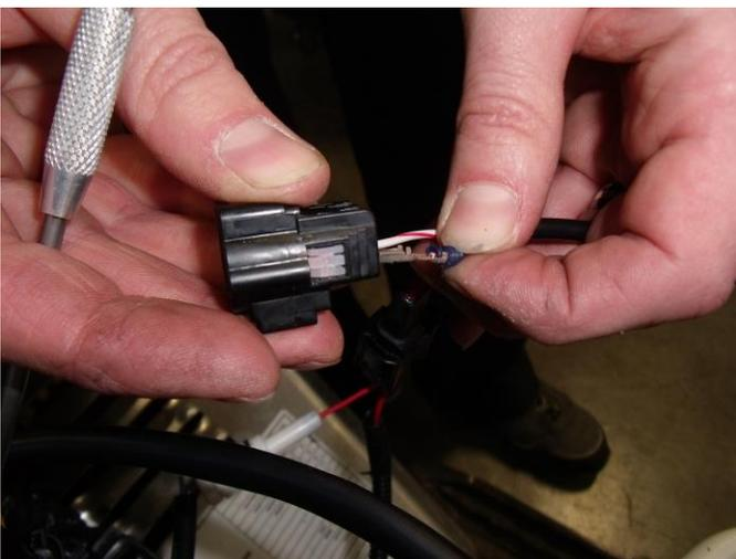
11. Once pins are removed located the black connector on the harness that has no wires inserted.
