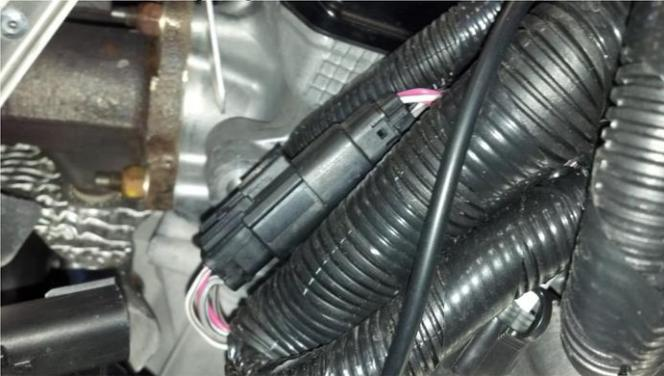
5. Plug matching EJK Harness into Factory injector harness.
