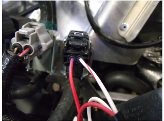
13. Plug the assembled connector into the mating EJK connector.
