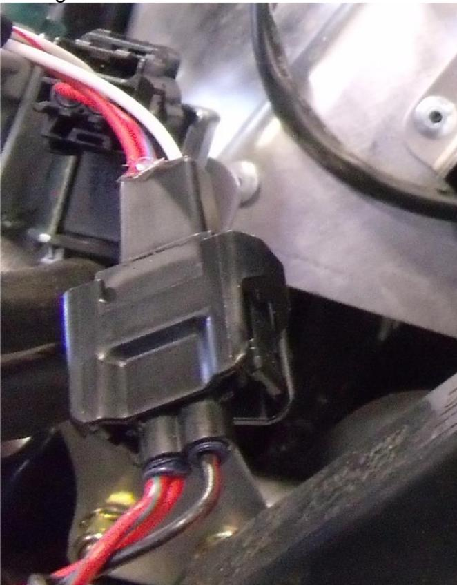
15. Plug connector back into Waste gate solenoid.
