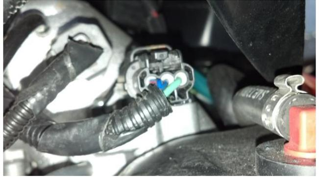
7. Unplug Stock Map sensor. Plug EJK Mating harness into factory harness and into the MAP sensor.
